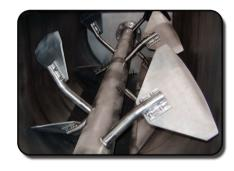
Suitable for mixing high viscous pastes or free flowing slurries, plastic pellets, cement, pigments and mud. The paddles lift and traject material in a folding/kneading like motion
